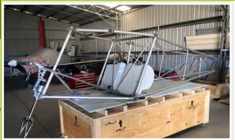
Study the manual and getting to grips with the methodology. Unwrapped the parts and checked if it corresponds with the manual. All parts are numbered in Sections, which correspond to the drawing numbers, and really easy to follow. We spend about 6 hours building today, and basically Completed the fuselage frame.
