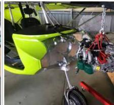
The engine, plus the subframe, was installed on to the main frame by means of the engine mounts.
