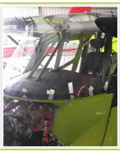
Installed the windshield, doors and finalised all the wiring to switches.
