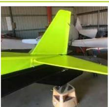
Most of today was spend covering the empennage parts and installing horizontal stabiliser, elevator and fitting cross bracing of cables etc.
