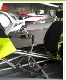
The main canopy fairing is now fitted, control stick is in, flap handle and rods fitted and seatbacks and harnesses all fitted.
