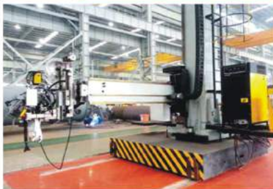
↑ ESAB窄间隙焊接工作站 ESAB Narrow Gap Welding Work Station
