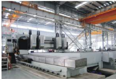
↑ DM7050、4B高速数控平面钻 (φ60 × 300mm) DM7050/4B CNC High Speed Plane Drilling Machine
