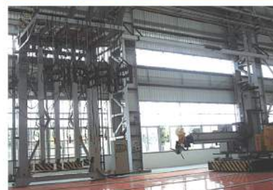
↑ DN4000整体多层夹套式包扎机 DN4000 Integrated Multi-layered Clamping and Wrapping Machine
