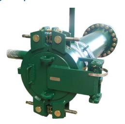
A Pig Trap is a pressure vessel. If installed at the ends of a pipeline allows the sending and reception of pistons used to clean the inside of the piping by scraping.
